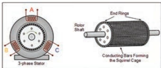
Figure 1: Squirrel Cage Induction Generator<sup>2</sup>
