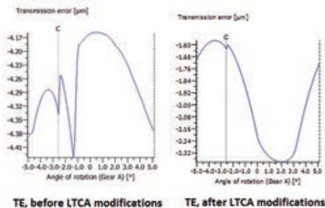
Figure 4: Transmission Error Analysis
