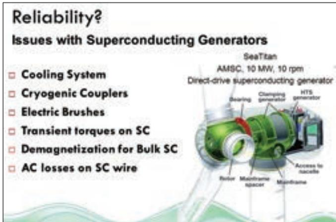
Figure 3: Issues with Superconducting Generators<sup>5</sup>
