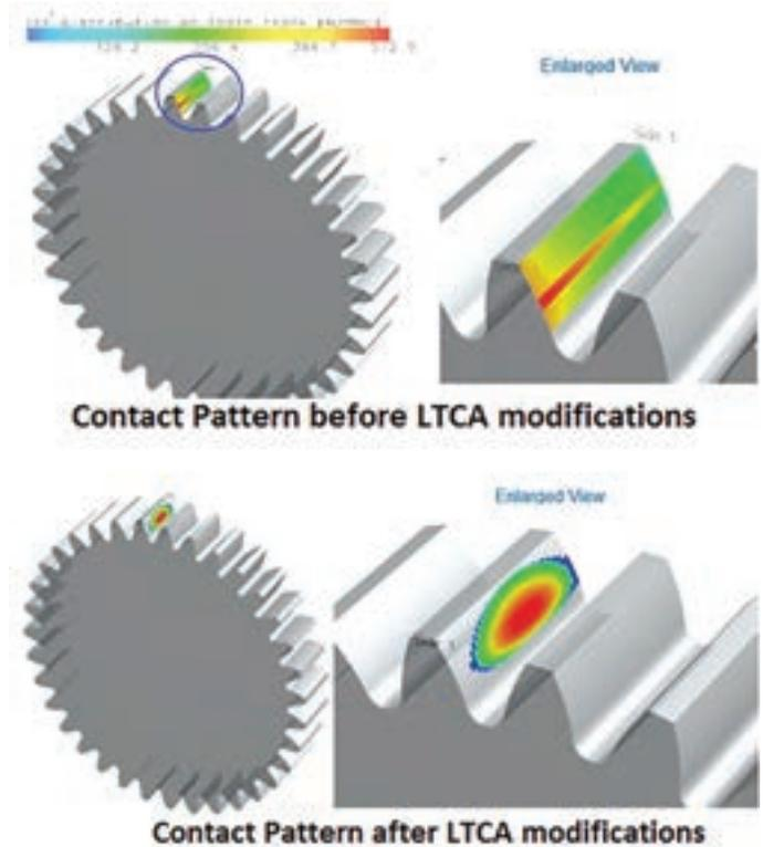
Figure 5: Simulated Contact Pattern with LTCA Design Parameters
