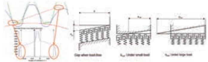
Figure 1: Tooth Pair in Contact as a Spring Model
