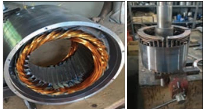
**Figure 3: Doubly Wound Stator and Specially Designed Rotor of 3.5 kW BDFIG Prototype Developed at Amrita Vishwa Vidyapeetham, Coimbatore**
