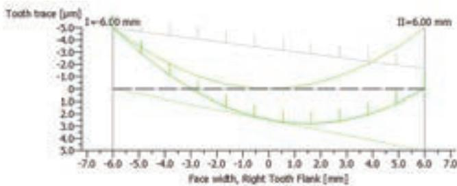
Figure 3: Profile and Lead modification curves thru LTCA Analysis
