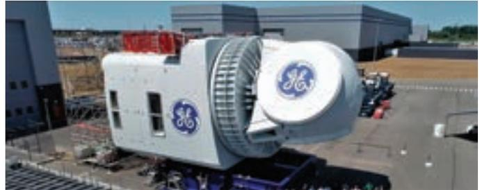
Figure 5: Nacelle of a 12 MW Wind Turbine<sup>7</sup>
