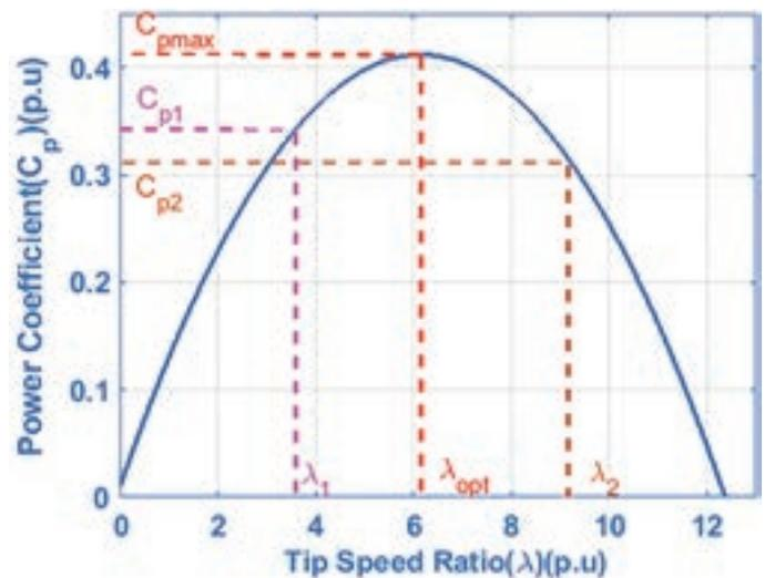
Figure 2: Typical Wind Turbine Characteristics
