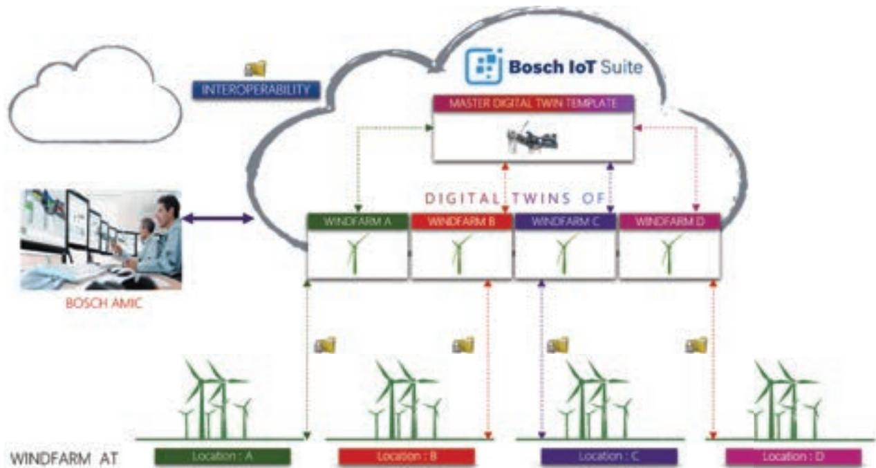
Figure 5: Digital Twin Deployment Method
