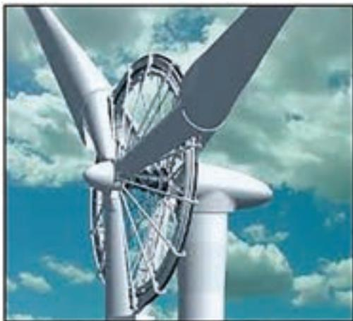
Figure 4: A 10 MW WEG with Ironless Stator Core<sup>6</sup>
