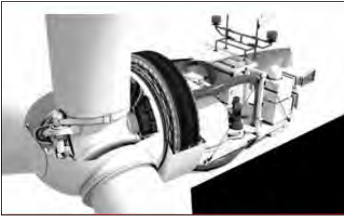
Figure 3: Direct Drive Wind Turbine 11
