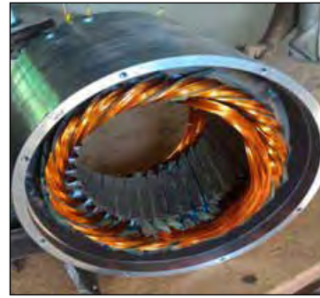
Figure 3: Stator Core with Two Windings
