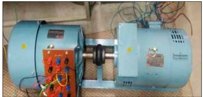
Figure 5(a): Prototype Model of BDFIM Coupled to DC Machine
